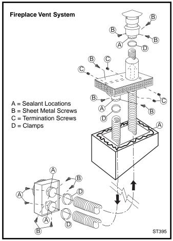
Fig. 35 Fireplace vent system installation.
